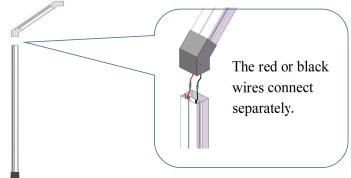
Step 2 Then, connect the other side of the sloped bar 600mm (with the cable entry) with the beam bar 2960mm, take out the wires of the sloped bar and the beam bar through the cable entry on the connectors, and screw it with self drilling screw;
