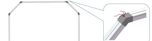
Step 5 assemble the panel light connectors and panel light as follow:
