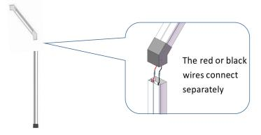
Step 4 Connect the parts of step2 & step3, take out the wires of the sloped bar and the beam bar through the cable entry on the connectors, and screw it with self drilling screw;
