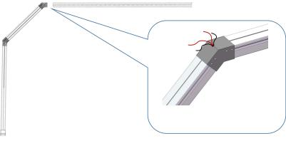
Step 3 as step1, connect another sloped bar 600mm (without the cable entry) with the post bar 2000mm, and screw it with self drilling screw;
