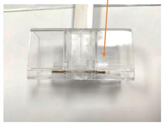
If two units do not seem to fit together easily, double check that the connectors are accurately lined up or try using a different lamp. Do not force the connection. Test the entire light set with a multimeter before hooking up to an electrical source and before mounting to the ceiling.
