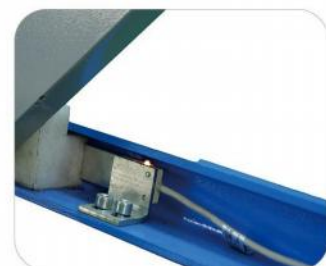
Limit device protects hydraulic cylinder
