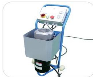
Separate control cabinet(24v) with equalizing system
